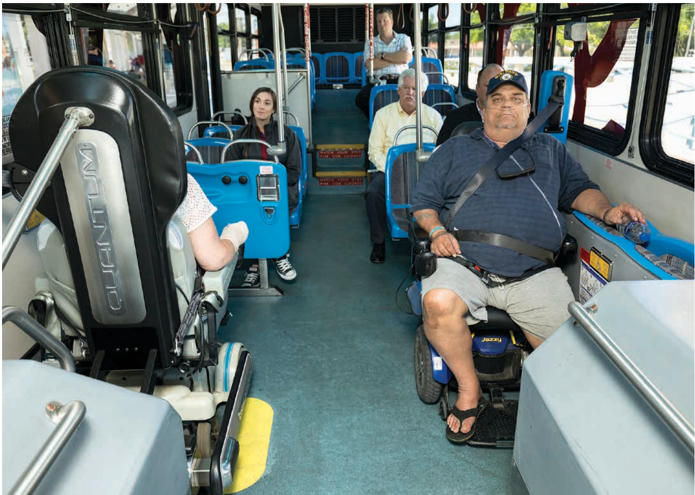
At right: Q’POD is the industry’s first fully integrated forward-facing wheelchair securement station specifically designed and tested for transit wheelchair passenger transportation.
