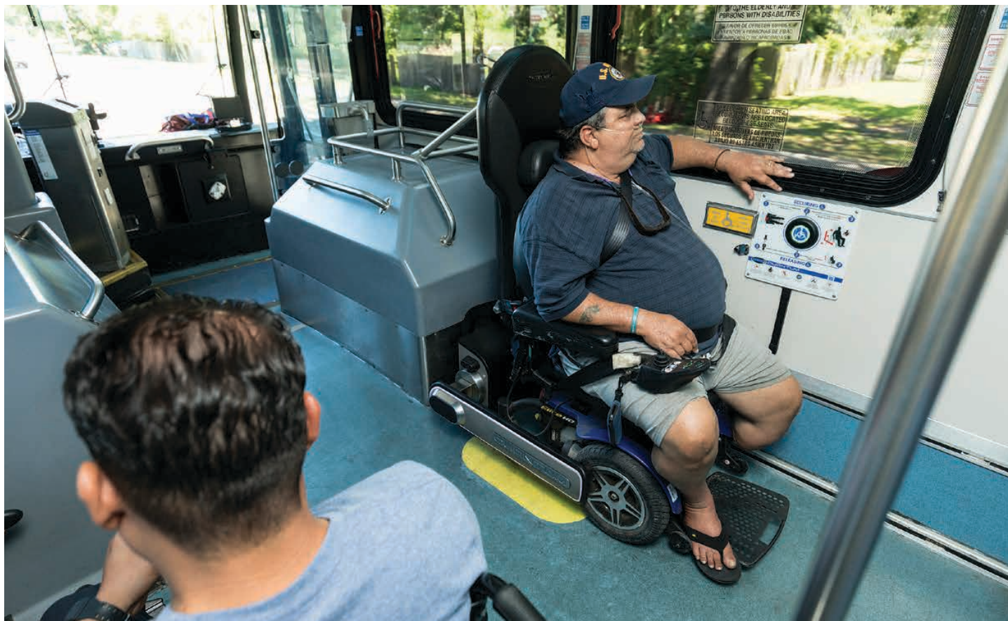
QUANTUM by Q'Straint is transit's first fully automatic rear-facing wheelchair securement station.
