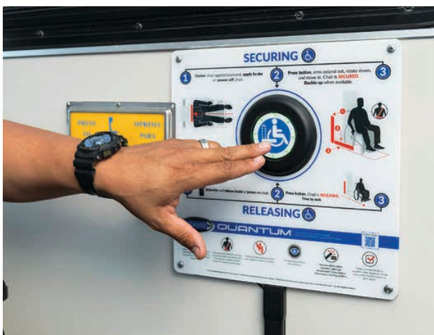
With QUANTUM, passengers can back their wheelchairs or scooters into the system, press a button and independently secure themselves.
